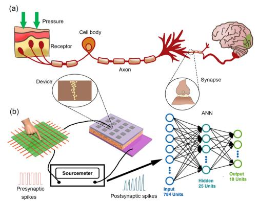
Fig. 4 (a) Schematic illustration of the biological tactile sensing system. (b) The artificial sensory neuron system consisting of tactile sensors, perovskite artificial synapses and ANNs.
