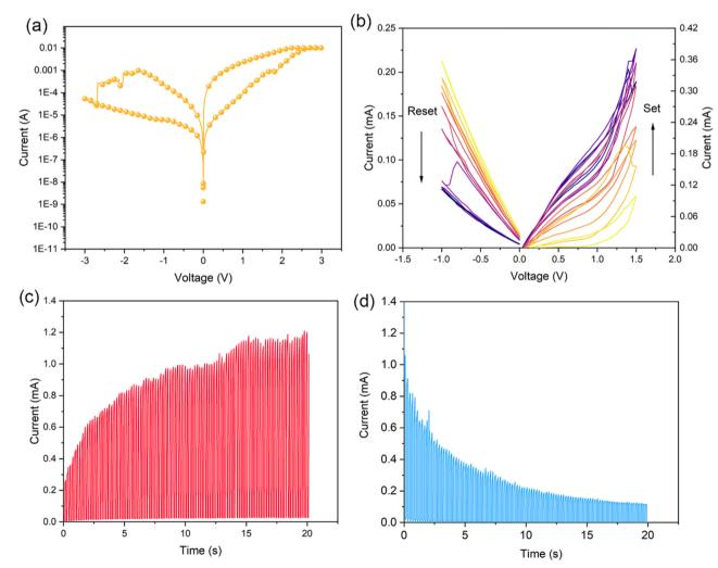
Fig. 2 (a) Typical current–voltage (I-V) curve of the AgBil<sub>4</sub> artificial synapse under positive and negative sweeps. (b) I-V curves under 10 positive and 10 negative voltage sweeps (0  $\rightarrow$  1.5  $\rightarrow$  0  $\rightarrow$  -1.0  $\rightarrow$  0 V). (c) The EPSC plasticity with positive pulses (1.5 V, 0.1 s). (d) The EPSC plasticity with negative pulses (-1.5 V, 0.1 s).
