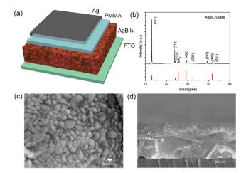
Fig. 1 (a) Schematic illustration of the AgBil<sub>4</sub> artificial synapse structure. (b) The experimental and reference (red lines) XRD patterns of the asprepared AgBil<sub>4</sub> perovskite layer. (c) The top-view SEM image of the AgBil<sub>4</sub> perovskite layer. (d) The cross-sectional SEM image of the whole device.
