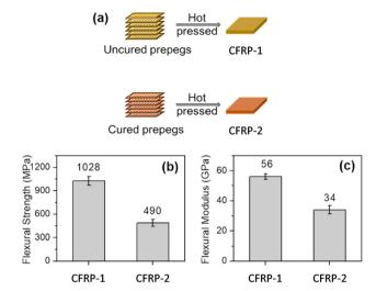
Fig. 6 Schematic fabrication of CFRP-1 and CFRP-2 composites (a); Comparison of the flexural strength (b) and modulus (c) of CFRC-1 and CFRC-2 composites. Modified with the permission of ref. 55. Copyright 2020 Elsevier Ltd
