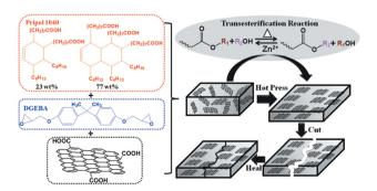
Fig. 10 Chemical structure of the monomers and the fabrication process of the aligned and healable graphene/epoxy composites. Reproduced with permission from ref. 68. Copyright 2019 Frontiers in Chemistry.
