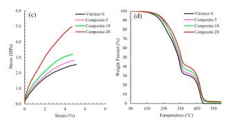
Fig. 17 (c) Tensile stress-strain curves and (d) TGA curves of Vitrimer-S and nanocomposites. Reproduced with permission from ref. 89. Copyright 2020 Elsevier Ltd.
