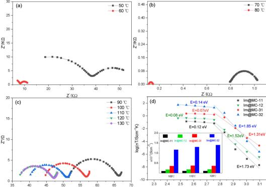
Fig. 5 AC impedance spectra of Im@MC-32 at different temperatures (a-c), and Arrhenius curves of the samples (d). The inset of (d) shows a comparison of the conductivity of the samples at different temperatures.
