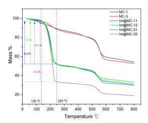
Fig. 4 Thermogravimetric curves of the samples under an  $\ensuremath{N_2}$  atmosphere.
