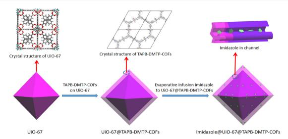
Scheme 1 Schematic of the synthetic route to imidazole@UiO-67@TAPB-DMTP-COFs.
