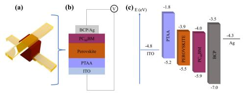
Fig. 1 MemPVCell schematic structure and energy bands. (a) Schematic illustration of the MemPVCell device having an inverted PSC structure and (b) consisting of a glass/ITO/PTAA/Perovskite/PC60BM/BCP/Ag material stack. (c) Graphic representation of the layer's energy diagram.
