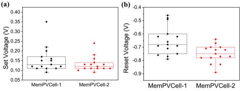
Fig. 5 Resistive switching voltage statistics for 15 MemPVCell-1 (black data) and 15 MemPVCell-2 devices (red data). MemPVCell-1 devices exhibit a slightly higher  $V_{\text{set}}$  while having a slightly lower  $V_{\text{reset}}$  compared to MemPVCell-2.  $I_{\text{cc}} = 10$  mA and a scanning rate of 10 mV s<sup>-1</sup> were used.
