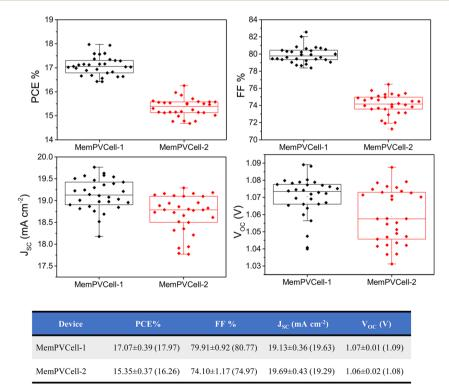
Fig. 2 Extraction of the photovoltaic parameters of the multiple MemPVCell-1 and MemPVCell-2 devices. Statistical variation of power conversion efficiency (PCE), fill factor (FF), short circuit current ( $J_{sc}$ ) and open circuit voltage ( $V_{oc}$ ) of 30 devices of each set.
