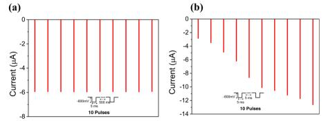
Fig. 11 Mimicking the spike-timing dependent plasticity (STDP) using a MemPVCell-1 device for 10 identical applied pulses (-600 mV of amplitude, 5 ms of duration) of (a) 500 ms and (b) 5 ms interval.
