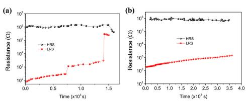
Fig. 8 Resistance state retention of (a) MemPVCell-1 and (b) MemPVCell-2. The following pulse settings were used: amplitude  $\pm 1$  V and pulse duration 500 ms. For resistance reading, a pulse with the amplitude of  $\pm 20$  mV and the duration of 10 ms every 5 s was used.
