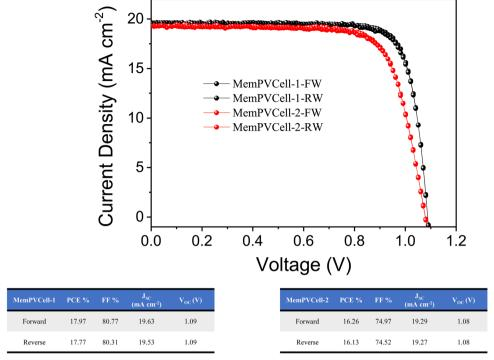
Fig. 3 J-V curves and photovoltaic parameters of champion devices of MemPVCell-1 and MemPVCell-2 for reverse and forward scan directions.
