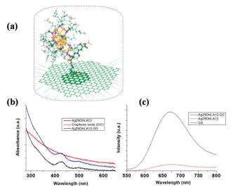
Fig. 19 Schematic view of the graphene oxide-nanocluster interface. (a) The nanocluster is Au<sub>15</sub>SR<sub>13</sub> (SR: thiolated molecules) covalently bound to graphene oxide. (b and c) absorption and emission spectra of silver nanoclusters electrostatically bound to graphene oxide nanosheets. adapted (Reproduced from ref. 187, with permission from [IOP Publishing, Ltdl).
