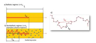
Fig. 3 Schematic of (a) ballistic and (b) non-ballistic regime (L is the size of the random medium (for example its length in 1D),  $L_G$  and  $L_A$  are the gain and amplification lengths receptively). (c) Representation of length scales ( $L_T$  and  $L_S$  are transport and scattering mean free paths respectively). ((a) and (b) is reproduced from ref. 31, with permission from [John Wiley and Sonsl)
