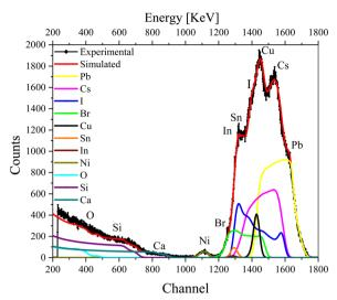
Fig. 4 RBS spectrum of the complete device excited from the Cu contact side, with simulation and deconvolution of the elemental spectra for glass/ ITO/NiOx/CsPbl2Br/C60/Cu.
