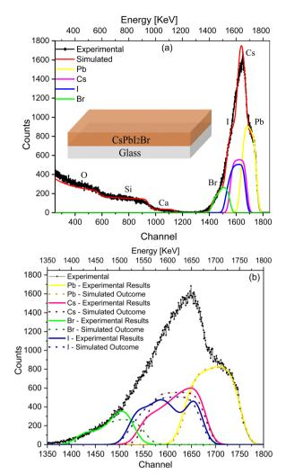
Fig. 2 (a) Simulated envelope of RBS in comparison with the experimental data for IHP (CsPbl $_2$ Br) deposited on glass. (b) Comparison of the elemental (I, Br, Cs, and Pb) spectra of the simulated envelope (dotted lines) and the experimental fitting envelope (solid lines).
