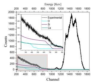
Fig. 5 RBS spectrum with quantification of oxygen in a complete device  $(glass/ITO/NiO/CsPbl_2Br/C_{60}/Cu)$ .
