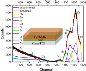
Fig. 3 RBS spectrum with the fitting of multilayer samples, i.e., glass/ITO/ NiO<sub>x</sub>/CsPbl<sub>2</sub>Br, excited from the IHP side, along with deconvolution of the elemental spectra
