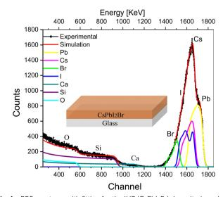
Fig. 1 RBS spectrum with fitting for the IHP (CsPbl<sub>2</sub>Br) deposited on glass, excited from the IHP side. The RBS spectrum is deconvoluted for various elements present in the film architecture, e.g., Pb, Cs, I, Br, Si, Ca, and O.
