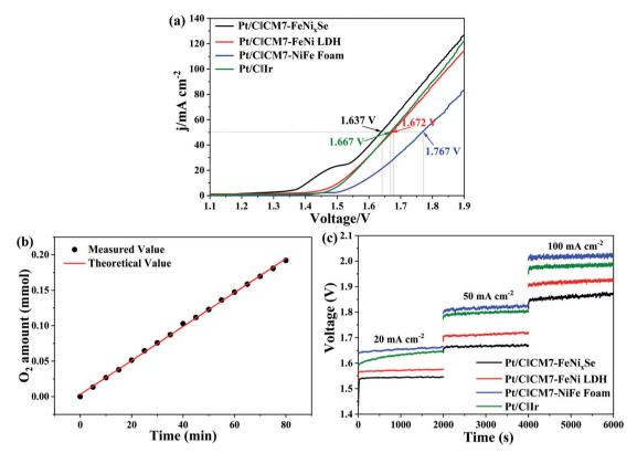
Fig. 6 (a) Polarization curves for overall water splitting. (b) Amounts of gas experimentally measured and theoretically calculated vs. time for the electrolyzer Pt/C∥CM7-FeNi,Se at 10 mA cm<sup>-2</sup>. (c) Chronopotentiometry curves tested at constant current densities of 10, 50 and 100 mA cm<sup>-2</sup>.
