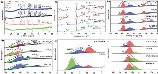
Fig. 2 (a) XRD patterns of NiFe foam, FeNi LDH, CM7-FeNi<sub>x</sub>Se and FeNi<sub>x</sub>Se. (b) XPS survey spectra and high-resolution XPS spectra of (c) Ni 2p, (d) Fe 2p, (e) Se 3d and (f) O 1s of NiFe LDH, CM7-NiFe LDH, CM7-FeNi<sub>x</sub>Se and FeNi<sub>x</sub>Se.
