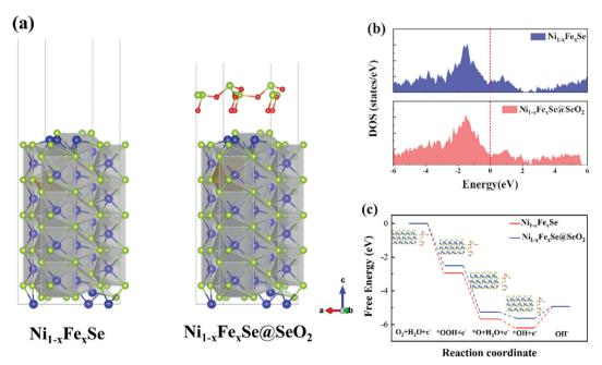
Fig. 5 Theoretical calculations of  $Ni_{1-x}Fe_xSe$  and  $Ni_{1-x}Fe_xSe@SeO_2$  electrocatalysts. (a) Crystal structures, (b) calculated DOS, (c) free energy diagram for the OER over four optimized adsorption geometry of O2, \*OOH, \*O, and \*OH.
