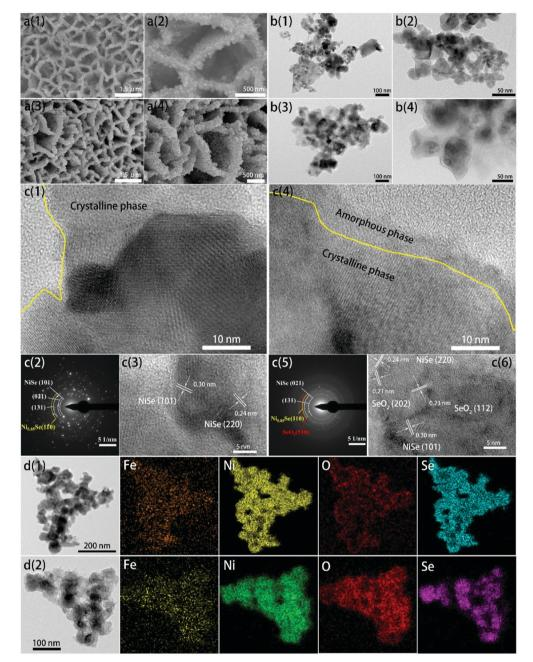
Fig. 1 (a1 and a2) SEM images, (b1 and b2) TEM images, (c1 and c3) HRTEM images, (c2) SAED pattern and (d1) EDX elemental mapping of FeNixSe; (a3 and a4) SEM images, (b3 and b4) TEM images, (c4 and c6) HRTEM images, (c5) SAED pattern and (d2) EDX elemental mapping of CM7-FeNi<sub>x</sub>Se.
