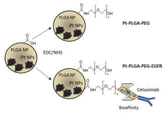
Fig. 8 Schematic representation of surface modifications performed on PLGA particles. Pegylated particles (Pt-PLGA-PEG) and antibody modified particles (Pt-PLGA-PEG-EGFR). B stands for biotin, N for neutravidin and Cetuximab is the commercial name of the monoclonal anti-EGFR antibody
