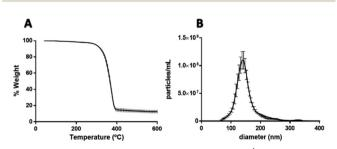
Fig. 7 (A) Thermogravimetric analysis of 0.015 mg  $\mu L^{-1}$  PtNPs with PLGA particles by nanoemulsion shows 12.5% weight percent loading of PtNPs. Performed 3 times with 3 different batches. (B) Size distribution by nanoparticle tracking analysis of 0.015 mg  $\mu L^{-1}$  PtNPs with PLGA particles by nanoemulsion. Shows a mode size of 140 nm.
