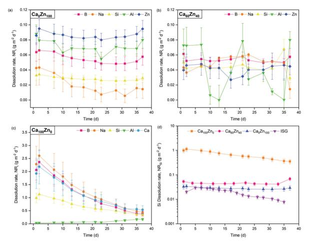
Fig. 9 Normalised dissolution rate (NR<sub>i</sub>) of elements released from the Ca<sub>x</sub>Zn<sub>y</sub> glass compositions during dynamic dissolution experiments. Showing (a)  $Ca_0Zn_{100}$ ; (b)  $Ca_{60}Zn_{40}$ ; (c)  $Ca_{100}Zn_0$ ; and (d) the  $NR_{Si}$  of all three  $Ca_xZn_y$  compositions investigated, compared with the International Simple Glass. 58.59 The scatter in Al data in (b) is attributed to the proximity of Al concentrations to the detection limit of the instrument.
