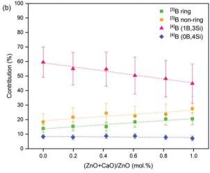
Fig. 7 Deconvolution of the  $^{11}B$  MAS NMR spectra for the  $Ca_xZn_y$  glass series. Showing (a) total  $^{[3]}B$  and  $^{[4]}B$  contribution; and (b) the proportion of individual  $^{[3]}B$  and  $^{[4]}B$  contributions.
