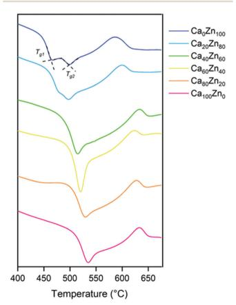
**Fig. 4** Differential thermal analysis traces for the  $Ca_xZn_y$  lithium alkaliborosilicate glass series, focussing on the glass transition range. The acquisition of  $T_g$  (°C) from linear extrapolation of the tangent points for  $Ca_0Zn_{100}$  is illustrated.
