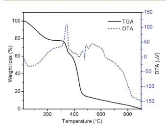
Fig. 1 TGA and DTA plots of PVP/metal nitrate composite nanofibers.
