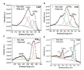
Fig. 5 High-resolution XPS spectra of LSCNO nanofibers: (a) La 4d; (b) Sr. 3d; (c) Ni 2d; and (d) Co 2p.
