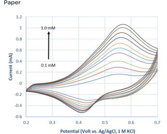
Fig. 7 Cyclic voltammograms of glucose on La<sub>0.75</sub>Sr<sub>0.25</sub>Co<sub>0.5</sub>Ni<sub>0.5</sub>O<sub>3</sub> nanofibers-modified carbon electrode: from bottom (blue) to top (dark purple) positive scans, the CVs represent 0.1, 0.2, 0.3, 04, 0.5, 0.6, 0.7, 0.8, 0.9, and 1.0 mM glucose, respectively. Initial potential: 0.2 V, Final Potential: 0.7 V, scan rate: 25 mV s<sup>-1</sup>
