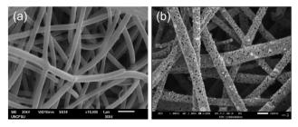
Fig. 3 SEM images of (a) PVP/metal salt precursor nanofibers before calcination, and (b) representative LSCNO nanofibers after calcination.
