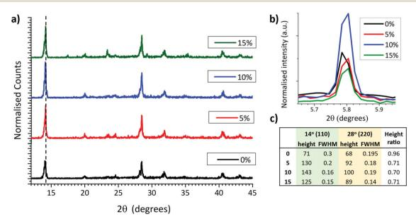
Fig. 3 (a) XRD of MAPbl<sub>3</sub> perovskites annealed from different GVL-MeOH solvent mixtures in inert mesoporous  $ZrO_2$  scaffolds.  $ZrO_2$  signals have been removed for clarity. (b) Magnified 2D peak at 5.8°. (c) Table showing peak heights, widths, and peak height ratios of the 14° (110) and 28° (220) signals.
