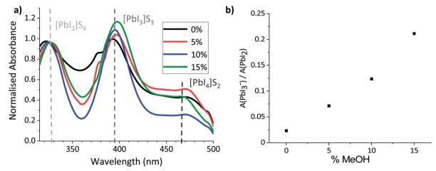
Fig. 2 (a) UV-Vis absorption spectra of MAPbl<sub>3</sub> in GVL-MeOH mixtures with 0, 5, 10 and 15% MeOH. It should be noted that the peaks at 380 nm in the 0 and 5% samples are caused by an equipment artefact and do not represent an absorption peak. (b) Change in height ratio of the Pbl<sub>2</sub> and Pbl<sub>3</sub><sup>-</sup> peaks with % MeOH.
