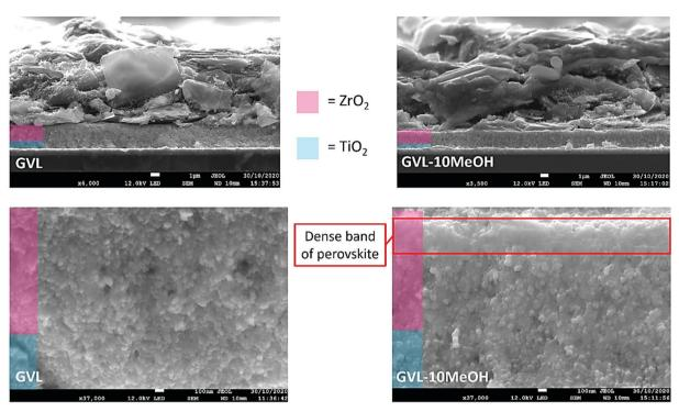
Fig. 6 Cross sectional images of devices made using GVL only or GVL-10MeOH. A dense band of perovskite is present at the ZrO<sub>2</sub>/C interface in the 10% samples (red box).
