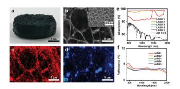
Fig. 2 (a) Photo of the as-prepared  ${\rm Ti_2O_3-PVA}$  sponge-like hydrogel sample. (b) SEM image of the sponge-like hydrogel and EDS mapping of (c) carbon and (d) titanium. (e) Absorption and (f) reflectance spectra in the wavelength range of 200–2000 nm. Reproduced with permission.  $^{24}$  Copyright 2019, American Chemical Society.
