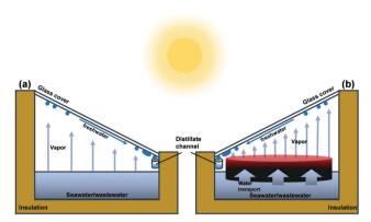
Fig. 1 Schematic illustrations of a single slope (a) solar still and (b) hydrogel based material platform for solar water purification.
