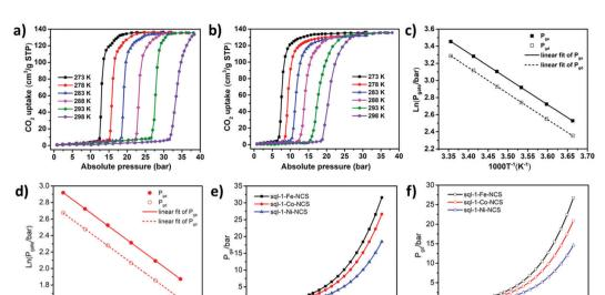
Fig. 3 High-pressure CO<sub>2</sub> sorption isotherms of (a) sql-1-Fe-NCS and (b) sql-1-Ni-NCS. The linear fit of gate sorption pressure (LnP) and temperature  $(1000 \text{ T}^{-1})$  using the Clausius-Clapeyron equation for (c) **sql-1-Fe-NCS** and (d) **sql-1-Ni-NCS**. (e) Calculated  $P_{\text{qa}}$  and (f)  $P_{\text{qd}}$  for **sql-1-M-NCS** (M = Fe,
