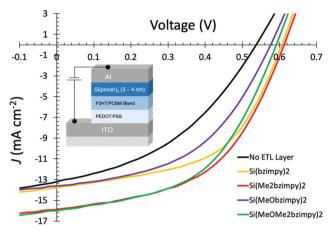
Fig. 6 Representative J-V measurement curves (with device structure inset image) of P3HT:PCBM OPV devices under 100 mW cm<sup>-2</sup> illumination with various Si(pincer)<sub>2</sub> electron transport layers (3–4 nm).
