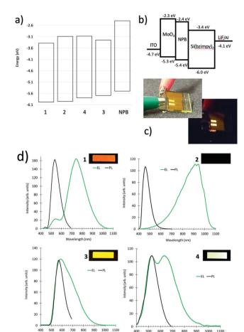
Fig. 5 Si pincer complex energy level comparisons (a), Si(bzimpy)<sub>2</sub> device construction with energy diagram (b), electroluminescence images (light and dark) from an encapsulated Si(bzimpy)<sub>2</sub> device (c), and overlaid photoluminescence and electroluminescence emission spectra of each Si pincer complex (d).
