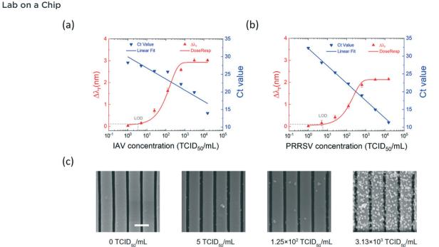
Fig. 5 Quantitative analysis of isolated IAV and PRRSV samples. (a) Measured  $\Delta \lambda_r$  as a function of isolated IAV concentration (red). The IAV titer was also measured using the RT-qPCR assay, and the Ct values were plotted (blue). (b) PC sensor response for the PRRSV titer (red) compared with the RT-qPCR Ct values (blue). (c) SEM images of the PC sensor surfaces after the adsorption of PRRSV-MNP at different PRRSV concentrations (scale bar: 555 nm).
