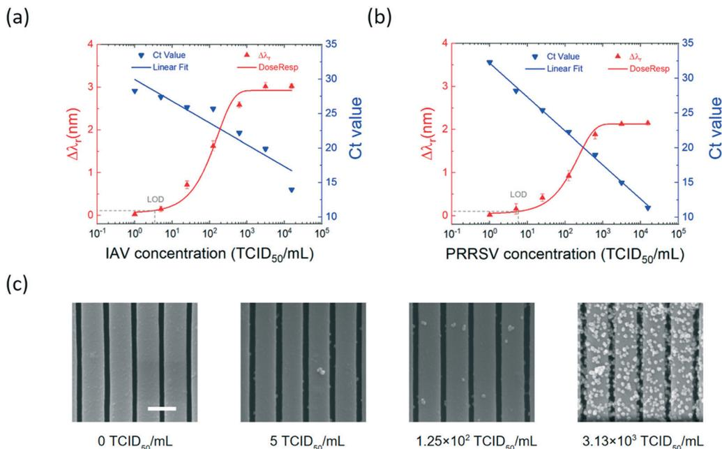
**Fig. 5** Quantitative analysis of isolated IAV and PRRSV samples. (a) Measured  $\Delta\lambda_r$  as a function of isolated IAV concentration (red). The IAV titer was also measured using the RT-qPCR assay, and the Ct values were plotted (blue). (b) PC sensor response for the PRRSV titer (red) compared with the RT-qPCR Ct values (blue). (c) SEM images of the PC sensor surfaces after the adsorption of PRRSV-MNP at different PRRSV concentrations (scale bar: 555 nm).
