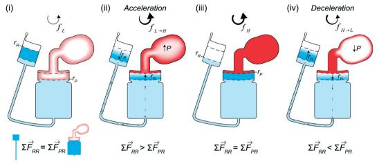
Fig. 2 Stages of CD LR. At a low rotation frequency (i) the forces acting on each column are equal  $(\vec{F}_{RR})$  and  $(\vec{F}_{RR})$  resulting in the liquid radial positions  $(\vec{F}_{RR})$  and  $(\vec{F}_{RR})$  and  $(\vec{F}_{RR})$  and the pressure in the GC to increase until the high rotation frequency (iii). Deceleration reverses the process (iv).
