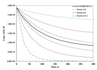
Fig. 5 Time-dependent concentration of a target compound with  $k_{\rm chem} = 1.0 \times 10^6 \, {\rm M}^{-1} \, {\rm s}^{-1}$  and different predicted values by a difference of a factor of 1.2, 2, and 5 in UV/sulfite process. 10
