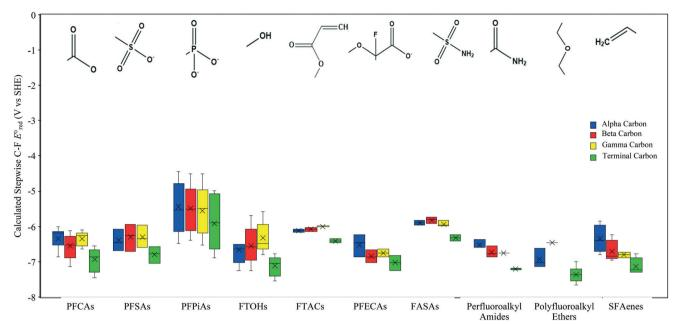
Fig. 4 Theoretically calculated  $E_{\text{red,aq}}^{\circ}$  values for the cleavage of a C-F bond at different positions of various PFASs. The  $E_{\text{red,aq}}^{\circ}$  values were calculated based on M06-2X/cc-pVDZ
