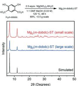
Fig. 3 PXRD ( $\lambda = 1.5406 \text{ Å}$ ) patterns of Mg<sub>2</sub>(m-dobdc)-ST synthesized on small and large scale under solvothermal conditions. The simulated pattern based on the previously reported single-crystal X-ray diffraction structure of the isostructural framework Co<sub>2</sub>(m-dobdc) is included for reference.25
