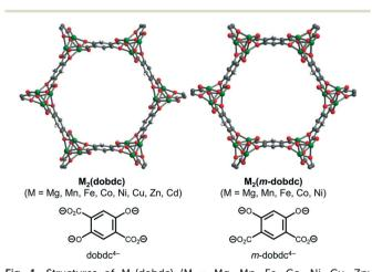
Fig. 1 Structures of  $M_2$ (dobdc) (M = Mg, Mn, Fe, Co, Ni, Cu, Zn;  $dobdc^{4-} = 2,5$ -dioxidobenzene-1,4-dicarboxylate, left) and  $M_2(m$ -dobdc)  $(M = Mq, Mn, Fe, Co, Ni; m-dobdc^{4-} = 4,6-dioxidobenzene-1,3$ dicarboxylate, right). Green, gray, white, and red spheres correspond to magnesium, carbon, hydrogen, and oxygen, respectively.
