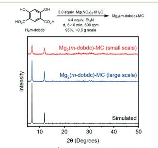
Fig. 4 PXRD ( $\lambda$  = 1.5406 Å) patterns of Mg<sub>2</sub>(m-dobdc)-MC synthesized on small and large scale under mechanochemical conditions. The simulated pattern based on the previously reported single-crystal X-ray diffraction structure of the isostructural framework Co<sub>2</sub>(mdobdc) is included for reference.<sup>25</sup>
