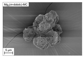
Fig. 5 SEM images of Mg<sub>2</sub>(m-dobdc)-ST (left) and Mg<sub>2</sub>(m-dobdc)-MC (right).
