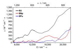
Fig. 2 UV-vis-NIR spectra of [U(TMP)<sub>2</sub>Bn<sub>2</sub>K(toluene)] (6U, black line) in THF (0.97 mM), and [Np(TMP)2Bn2K(toluene)] (6Np, red line) in toluene (0.50 mM), and [Pu(TMP)<sub>2</sub>Bn<sub>2</sub>K(toluene)] (**6Pu**, blue line) in toluene (1.00 mM) between 7000-22 000 cm<sup>-1</sup> (1429-455 nm) at room temperature.
