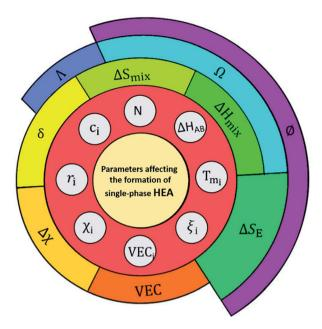
Fig. 4 Parameters affecting the formation of single-phase HEAs.
