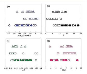
Fig. 2 Effect of (a)  $\Delta H_{\text{mix}}$ , (b)  $\delta$ , (c)  $\Delta \chi$ , and (d) VEC on phase stability in HEAs. The symbols  $\Box$ ,  $\Delta$ ,  $\bigcirc$  and  $\bigcirc$  represent the solid solution phase, intermetallic phase, equimolar amorphous phase, and non-equimolar amorphous phase, respectively. Reproduced with permission (ref. 40). Copyright 2011, Elsevier.
