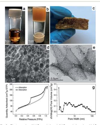
Fig. 2 Photographs of (a) Fe-gelatin sol, (b) Fe-gelatin gel and (c) Fegelatin aerogel after freeze-drying treatment; (d) SEM and (e) TEM images, (f) nitrogen adsorption and desorption isotherms and (g) corresponding pore size distribution of FCA2.
