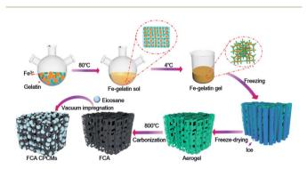
Fig. 1 Schematic of the synthesis of the FCA PCM composites.
