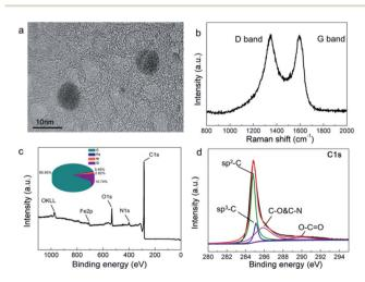
Fig. 3 (a) High resolution TEM image, (b) Raman spectrum, (c) XPS spectrum and (d) C1s spectrum of FCA2
