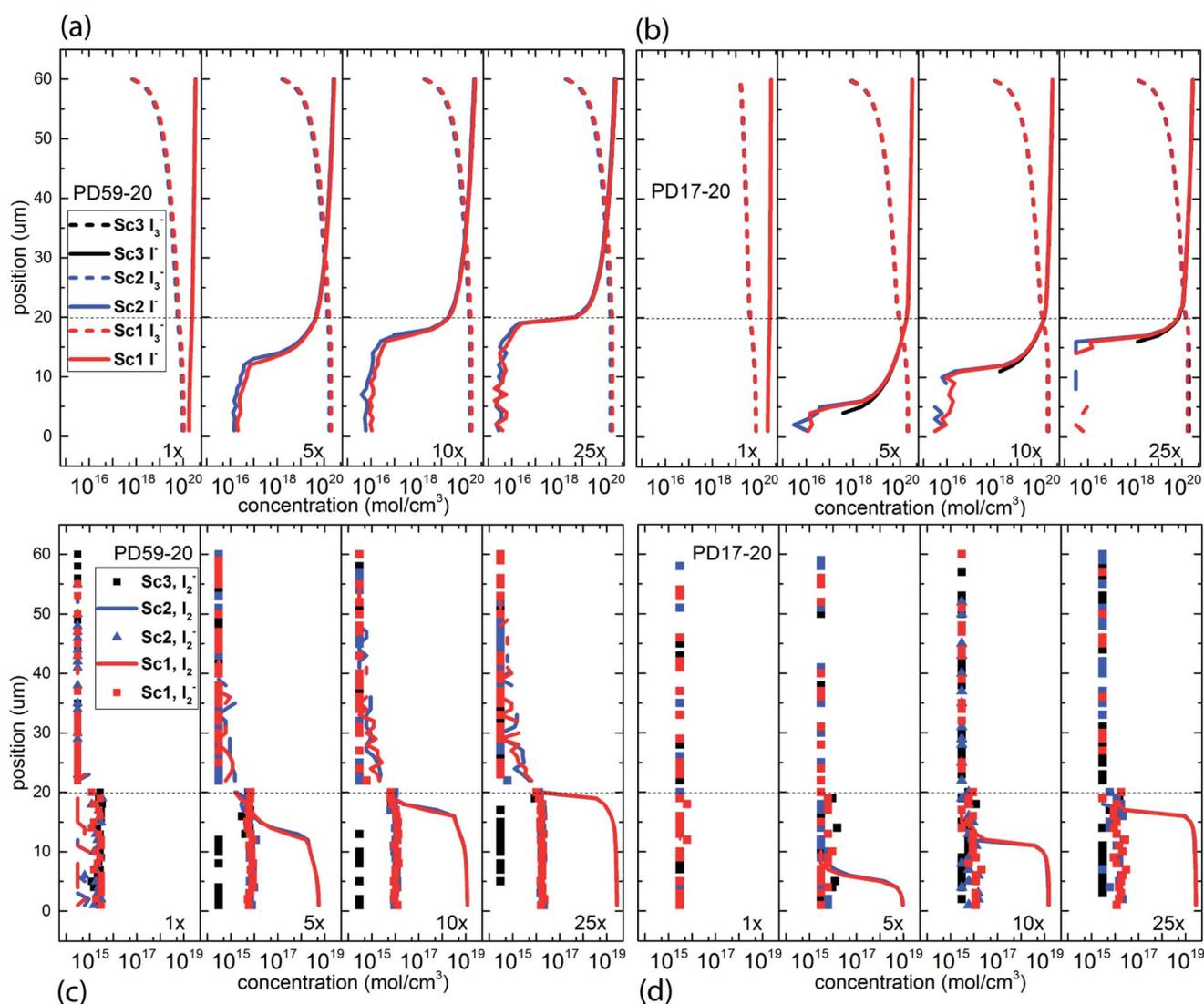
Fig. 3 Electrolyte composition at 0.8 s (close to steady state) as a function of position within the system. The photoanode contact is at 0 μm, the interface between the photoanode and bulk electrolyte is at 20 μm, and the cathode is at 60 μm. (a)  $\text{I}^-$  and  $\text{I}_3^-$  profiles for PD59-20, (b)  $\text{I}^-$  and  $\text{I}_3^-$  profiles for PD17-20, (c)  $\text{I}_2^-$  and  $\text{I}_2$  profiles for PD59-20, (d)  $\text{I}_2^-$  and  $\text{I}_2$  profiles for PD17-20.
