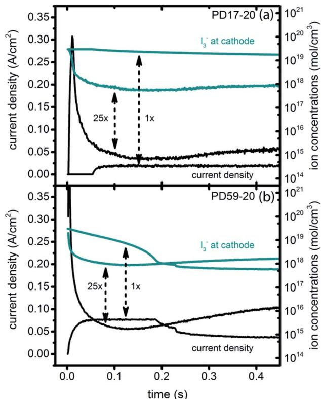
Fig. 9 Current transients (left axis) and  $I_3^-$  concentrations at the cathode (right axis) for Sc2. (a) PD17-20, 1 $\times$  and 25 $\times$  excitation frequencies; (b) PD59-20, 1 $\times$  and 25 $\times$  excitation frequencies.
