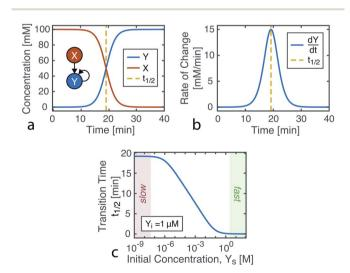
Fig. 1 Kinetics of autocatalysis. (a) Reagent and autocatalytic product evolution over time for  $X_0 = 100$  mM,  $Y_0 = 1 \mu$ M, and k = 0.1 (eqn (4)). (b) Rate of product concentration change over time for the reaction simulated in a, showing the accelerated production typical of an autocatalytic process. (c) The time to transition as the input catalyst concentration ( $Y_o$ ) is varied about a constant:  $Y_o = Y_i + Y_s$  with  $Y_i = 1$  $\mu$ M,  $X_0 = 100$  mM, and k = 0.1.
