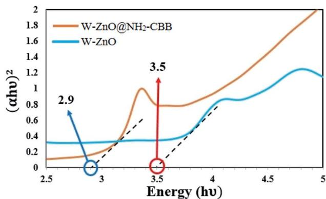
Fig. 7 Optical band-gap analysis of W-ZnO@NH<sub>2</sub>-CBB and W-ZnO.
