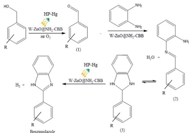
Scheme 2 A suggested mechanism for the synthesis of 2-substituted benzimidazoles catalyzed by W-ZnO@NH<sub>2</sub>-CBB.
