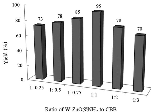
Fig. 11 Effect of W-ZnO@NH<sub>2</sub>:CBB ratio on the efficacy of condensation reaction. Reaction condition is similar to that in the caption of Fig. 8. Reaction time was 2 h. 0.02 g of photocatalyst was used in all cases.
