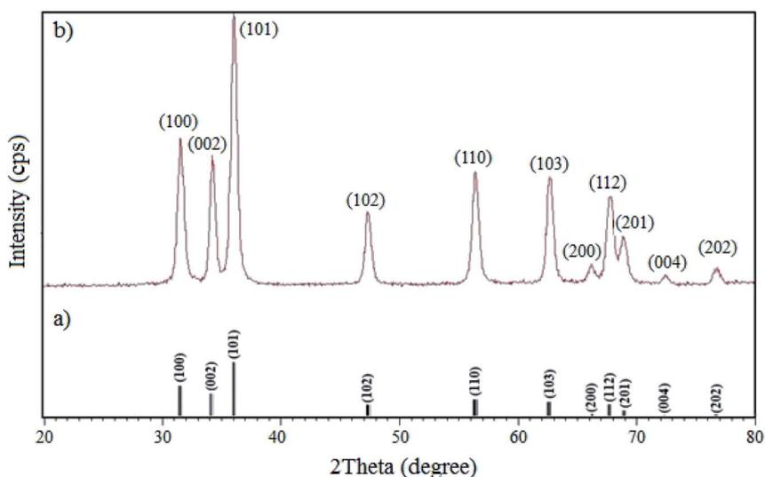
Fig. 5 XRD patterns of (a) simulated standard ZnO and (b) real W-ZnO@NH<sub>2</sub>-CBB.
