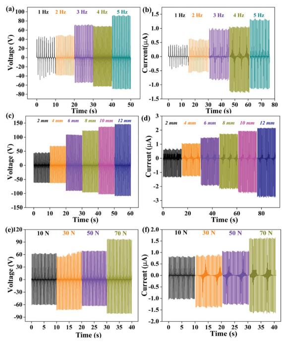
Fig. 4 (a) and (b)  $V_{oc}$  and  $I_{sc}$  of DL<sub>1</sub>/DL<sub>2</sub> TENG with various frequencies (1–5 Hz); CS distance and load were fixed at 4 mm, and 50 N, (c) and (d)  $V_{oc}$ and I<sub>sc</sub> evaluation under different CS distances (2 to 12 mm) with a constant load of 50 N and frequency of 4 Hz, (e) and (f) shows the performance of  $V_{oc}$  and  $I_{sc}$  for different contact forces (10–70 N) with a constant frequency and CS distance (4 Hz and 4 mm).
