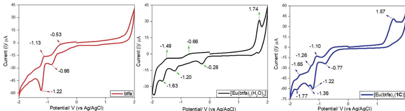
Fig. 7 Cyclic voltammograms of btfa (red),  $[\text{Eu}(\text{btfa})_3(\text{H}_2\text{O})_2]$  (black) and  $[\text{Eu}(\text{btfa})_3]1\text{c}$  (blue) in the region between  $-2.0$  to  $2.0$  V on glassy carbon electrode in  $0.1$  M  $\text{Bu}_4\text{NPF}_6$  solution in DCM at a scan rate of  $100$   $\text{mV s}^{-1}$ .
