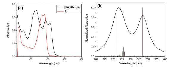
Fig. 2 (a) Optical absorption spectra of 1c and [Eu(btfa)<sub>3</sub>1c] at RT. (b) Theoretical electronic spectrum calculated at the CAM-B3LYP level of theory using the B3LYP geometry for [Eu(btfa)<sub>3</sub>1c].
