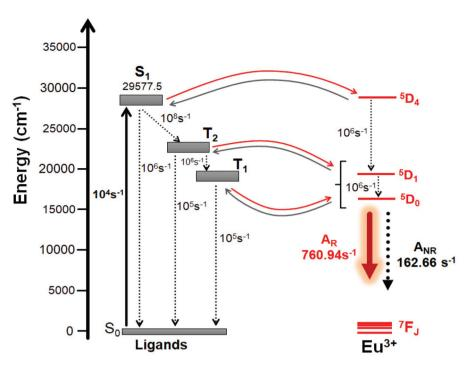
Fig. 6 Schematic energy-level diagram showing the most important ET channels for [Eu(btfa)<sub>3</sub>1c]. Please see Table 5 for the corresponding values of ET rates.
