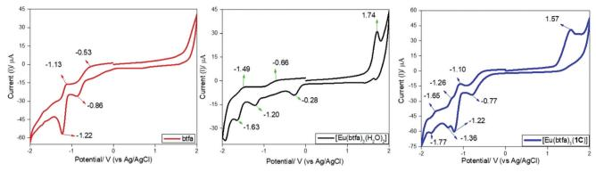
Fig. 7 Cyclic voltammograms of btfa (red), [Eu(btfa)<sub>3</sub>(H<sub>2</sub>O)<sub>2</sub>] (black) and [Eu(btfa)<sub>3</sub>1c] (blue) in the region between -2.0 to 2.0 V on glassy carbon electrode in 0.1 M Bu<sub>4</sub>NPF<sub>6</sub> solution in DCM at a scan rate of 100 mV s<sup>-1</sup>.
