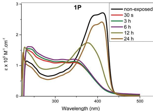
Fig. 6 Absorption spectral profile of **1P** prior to exposure (non-exposed) and measured at different intervals for the recovery process of the initially exposed sample to 25 minutes irradiation at 365 nm.
