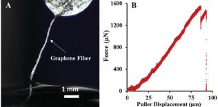
Fig. 3 Macroscale graphene fiber tested in uniaxial tension. (A) Optical image of graphene fiber ( $A_{graphene} = 3.18 \mu m^2$ ,  $L_{fiber} = 2952 \mu m$ ). (B) Forcedisplacement plot of uniaxial tensile test (puller displacement rate  $r_p = 0.50 \,\mu\text{m s}^{-1}$ ). This fiber exhibited brittle fracture, with a tensile strength of 0.475 GPa.
