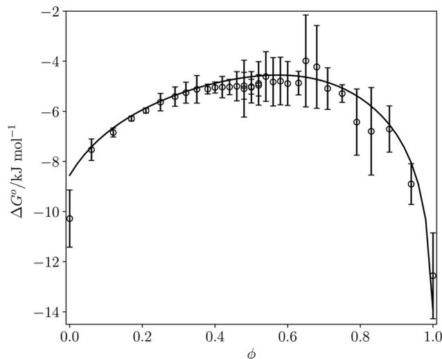
Fig. 12  $\Delta G^\circ$  ( $\text{kJ mol}^{-1}$ ) for formation of a 1 : 1 complex between tri-*n*-butylphosphine oxide ( $\beta = 10.7$ ) and 4-phenyl azophenol ( $\alpha = 4.1$ ) in THF–chloroform mixtures. Experimental measurements (black circles) and calculated values using eqn (16) (black line) as function of chloroform volume fraction,  $\phi$ . The experimental values are the average of five experiments with error bars at the 95% confidence limit.
