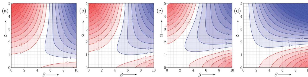
Fig. 10 FGIPs for the interaction of two solutes in (a) 100% THF 0% chloroform (b) 70% THF 30% chloroform (c) 30% THF 70% chloroform (d) 0% THF 100% chloroform mixtures by volume at 298 K ( $\Delta\Delta G_{\text{FGI}}$  in  $\text{kJ mol}^{-1}$ ). The solute–solute interactions are favourable in the blue region, and unfavourable in the red region.
