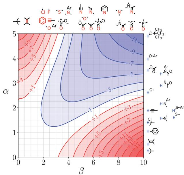
Fig. 8 FGIP for the interaction of two solutes in heptanoic acid at 298 K ( $\Delta\Delta G_{\text{FGI}}$  in  $\text{kJ mol}^{-1}$ ). The solute-solute interactions in the blue region, and unfavourable in the red region.
