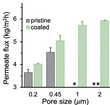
Fig. 7 Permeate flux of PP membranes before and after 8 min of PHDFA coating using high-salinity feed with  $100 \text{ g L}^{-1}$  NaCl. The pristine 1 and  $2 \text{ }\mu\text{m}$  membranes leaked during MD while the coated membranes remained nonwetted. \* and \*\* indicate intermittent and frequent leaking, respectively.
