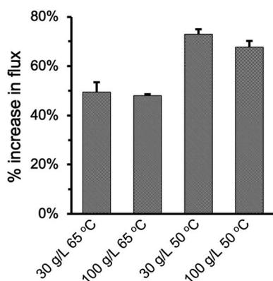
Fig. 8 Percentage increase in the permeate flux under different operation conditions when the nominal pore size increases from  $0.2 \text{ }\mu\text{m}$  to  $2 \text{ }\mu\text{m}$  for PP membranes after 8 min of PHDFA coating.
