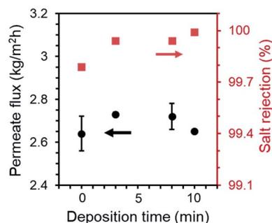
Fig. 5 Permeate flux and salt rejection of 0.45 μm PP membranes after PHDFA coating with varying deposition time. Test condition: feed temperature at 50 °C, flow rate at 0.81 L min<sup>-1</sup>, NaCl concentration at 30 g L<sup>-1</sup>.
