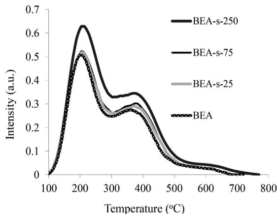
Fig. 7  $\text{NH}_3$ -TPD curves of synthesized BEA zeolites.
