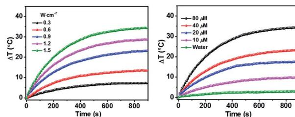
Fig. 3 Photothermal property of **HSA- $\alpha$ -Pc** NPs in aqueous solution under 808 nm laser irradiation. Left: Light intensity-dependent temperature increase at the concentration of 80  $\mu\text{M}$  (Pc equiv.). Right: Concentration-dependent temperature increase with a 0.9  $\text{W cm}^{-2}$  laser intensity.
