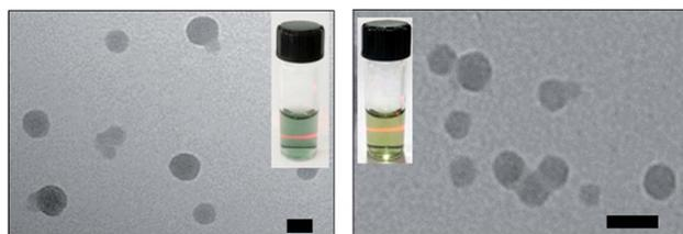
Fig. 2 TEM images of **HSA- $\alpha$ -Pc** NPs (left) and **HSA- $\beta$ -Pc** NPs (right), scale bars: 50 nm. The insets present the picture of their Tyndall phenomenon in aqueous solution, which further supports the TEM and DLS analysis.
