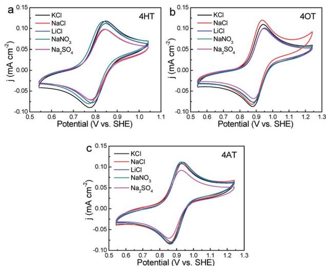
Fig. 3 CVs of 1 mM 4HT (a), 4OT (b) and 4AT (c) in different supporting electrolytes (0.5 M) at a scan rate of 25 mV s<sup>-1</sup>, respectively.
