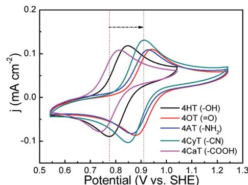
Fig. 1 CV curves of five TEMPO derivatives (1 mM) in 0.5 M KCl supporting electrolyte (pH = 7) at a scan rate of 25 mV s $^{-1}$  at 25  $^{\circ}$ C. Before CV measurements, the pH values of the electrolyte solutions were adjusted to 7 for 4AT and 4CaT by using 0.01 M HCl and KOH solution, respectively, because 4AT is weakly alkaline and 4CaT is weakly acidic.
