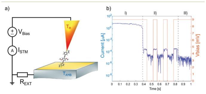
Fig. 3 (a) STM break junction setup for the electric and thermoelectric characterization of single molecules; (b) typical example of opening trace: I(t) and  $V_{\text{bias}}(t)$  for a single-molecule junction.
