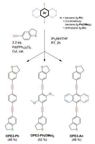
Fig. 1 Synthesis of the OPE3 derivatives.
