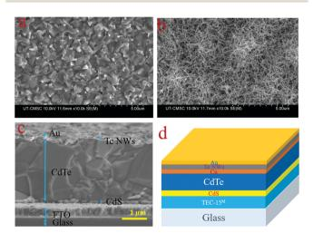
Fig. 4 SEM images of  $CdCl_2$  treated CdTe (a) top surface w/o Te NWs and (b) top surface with Te NWs (c) cross-sectional image with Te NWs as HTL and (d) schematic diagram of the device structure.
