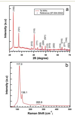
Fig. 3 (a) X-ray diffraction pattern of synthesized Te NWs obtained from  ${\rm TeO_2}$ , possess hexagonal crystal structure and the sharp intensity peaks of the pattern indicate pure-phase crystalline material. The reference lines (PDF #97-004-0042) was obtained from MDI JADE software, and (b) Raman spectroscopy measurement of Te NWs using a 632.8 nm excitation from a He–Ne laser with 0.1 gm PVP and 0.75 mL ascorbic acid.
