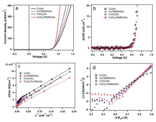
Fig. 6 Analysis of dark J-V curves with back contacts Cu/Au, Cu/TeNWs/Au, CuCl<sub>2</sub>/Au and CuCl<sub>2</sub>/TeNWs/Au (a) dark J-V curve (b) shunt characterization (c) plot of dV/dJ versus l/J for calculation of A and  $R_s$  (d) plot of ln(J) versus  $V-R_sJ$  for calculation of n and  $J_0$ . The solid lines represent the corresponding fitted lines in (c) and (d).
