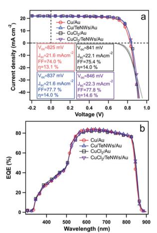
Fig. 5 (a) J-V characteristics and (b) external quantum efficiency (EQE) of CdTe solar cells with Cu/Au, Cu/TeNWs/Au, CuCl<sub>2</sub>/Au and CuCl<sub>2</sub>/TeNWs/Au back contacts respectively. The solid and dotted lines in Fig. 5(a) represent J-V curves under illumination and dark conditions respectively.
