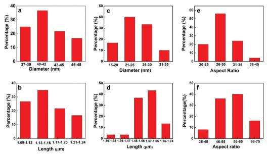
Fig. 2 Diameter, length and aspect ratio distribuiton of Te NWs at 120 °C for 21 h. (a), (b) and (e) 0.1 g PVP and 0.75 mL ascorbic acid (c), (d) and (f) 0.2 g PVP and 1.5 mL ascorbic acid.
