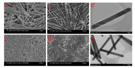
Fig. 1 SEM images of Te NWs obtained from TeO<sub>2</sub> with ethylene glycol at 120 °C (a) and (b) 0.1 gm PVP and 0.75 mL ascorbic acid (c) and (d) 0.2 gm PVP and 1.5 mL ascorbic acid and (e) and (f) STEM images of Te NWs obtained from 0.1 gm PVP and 0.75 mL ascorbic acid.
