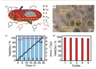
Fig. 4 (a) Schematic representation of nickel-decorated ultrathin CdS nanosheets as photocatalysts for the C–N coupling of amines to imines. (b) HRTEM of the Ni/CdS photocatalyst. (c) Photocatalytic performance of Ni/CdS for the production of imines and H<sub>2</sub> during photolysis. (d) Stability test of Ni/CdS for five consecutive photolysis experiments. Reprinted from ref. 36 with permission from American Chemical Society, copyright 2020.
