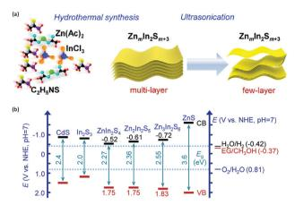
Fig. 3 (a) Schematic illustration of the low-temperature hydrothermal and ultrasonic process used to synthesize  $Zn_m ln_2 S_{m+3}$ . (b) Energy levels of several related redox couples and band-edge positions of selected semiconductors. Reprinted from ref. 32 with permission from Royal Society of Chemistry, copyright 2020.
