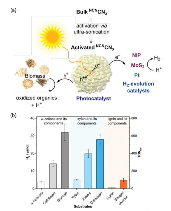
Fig. 6 (a) Schematic photo-reforming of lignocellulose using  $^{\rm NCN}{\rm CN}_{\rm x}$  and proton reduction co-catalysts. (b) Photocatalytic H<sub>2</sub> production from purified lignocellulose components catalyzed by activated  $^{\rm NCN}{\rm CN}_{\scriptscriptstyle X}$  and NiP under AM1.5G light irradiation for one day at 25 °C. Reprinted from ref. 48 with permission of American Chemical Society, copyright 2018.
