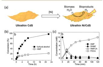
Fig. 2 (a) Synthetic route of ultrathin Ni/CdS nanosheets for integrated H<sub>2</sub> production and biomass valorization. (b) Concentration change over time for the photocatalytic oxidation of furfural alcohol and HMF under neutral conditions. (c) Concentration change over time for the photocatalysis of HMF under alkaline conditions. Reprinted from ref. 30 with permission from American Chemical Society, copyright 2017.
