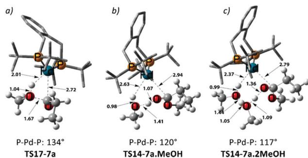
**Fig. 1** 3D representations of selected transition states. Distances are given in Å. Additional methanol units acting as a relay in this transition state alleviate strain on the P–Pd–P bite angle and facilitate methanolysis.
