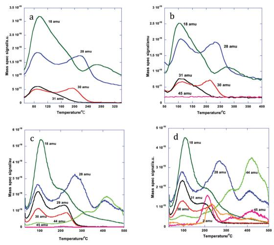
Fig. 3 Desorption products during TPD from the doped HSA Fe<sub>2</sub>O<sub>3</sub> samples, coated with 3 ML equivalent of MoO<sub>y</sub>: (a) 5% Al doped, (b) 10%, (c) 15% and (d) 20%.
