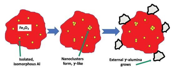
Fig. 7 Showing the evolution of the structure when doping Al into haematite. First the Al is substituted in the lattice with the same corundum structure as the iron oxide. Then small nanoclusters begin to form within the haematite nanoparticles. Finally separated alumina nanocrystals begin to form.
