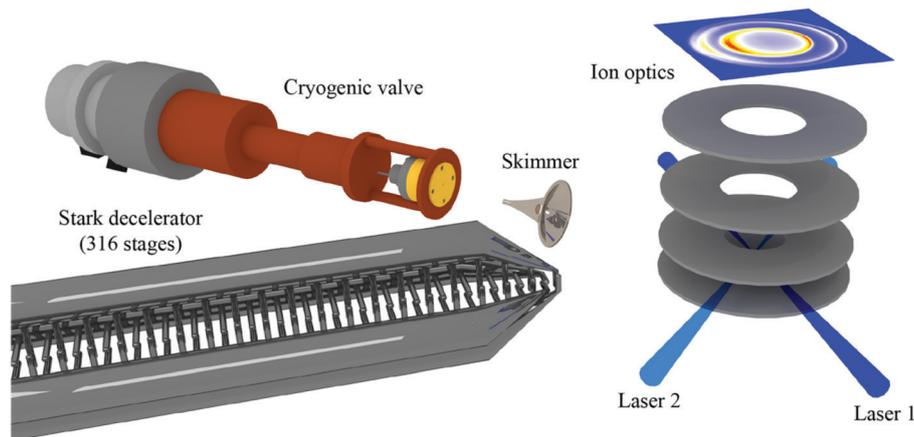
Fig. 1 Schematic representation of a crossed beam apparatus. A beam of NO radicals is passed through a Stark decelerator and scattered with a pulsed beam of *para*-H<sub>2</sub> or *ortho*-D<sub>2</sub>. The inelastically scattered NO radicals are state-selectively ionised using two pulsed lasers and detected using velocity map imaging. Only the last section of the Stark decelerator is shown. Reprinted with permission from Gao *et al.*,<sup>58</sup> copyright 2017 American Chemical Society.
