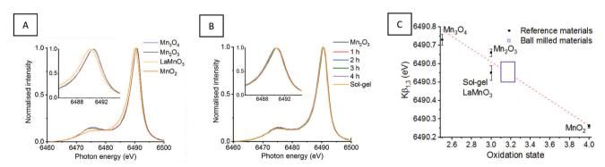
Fig. 2 Mn Kβ XES mainlines for (A) Mn reference oxides and sol–gel synthesised LaMnO<sub>3</sub> with (B) 'time-slices' during the mechanochemical synthesis of LaMnO<sub>3</sub> (C) presents the Kβ<sub>1,3</sub> max as a function of oxidation state, with a line of best fit calculated from the reference materials and used to calculate the oxidation state of the ball milled materials.
