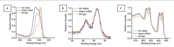
Fig. 9 XPS in the (A) O 1s, (B) Mn 3s and (C) La 3d region for LaMnO<sub>3</sub> synthesised by sol-gel and mechanochemistry with air and argon environments.
