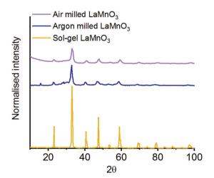
${\rm Fig.~5}~~{\rm XRD}$  patterns  ${\rm LaMnO_3}$  mechanochemically synthesised 4 h under atmospheric and inert (argon) conditions compared to the sol–gel synthesised perovskite.
