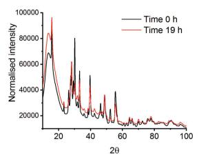
Fig. 3  $\,$  XRD patterns at time 0 h and time 19 h after milling La<sub>2</sub>O<sub>3</sub> and Mn<sub>2</sub>O<sub>3</sub> with a PMMA vibrational mill.
