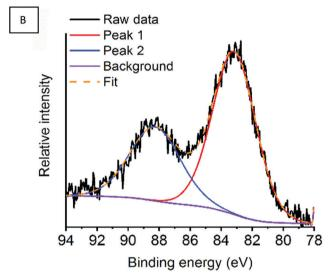
Fig. 11 (A) Mn 2p region and (B) Mn 3s region for the argon milled catalyst at RT under a  $N_2O$  atmosphere.
