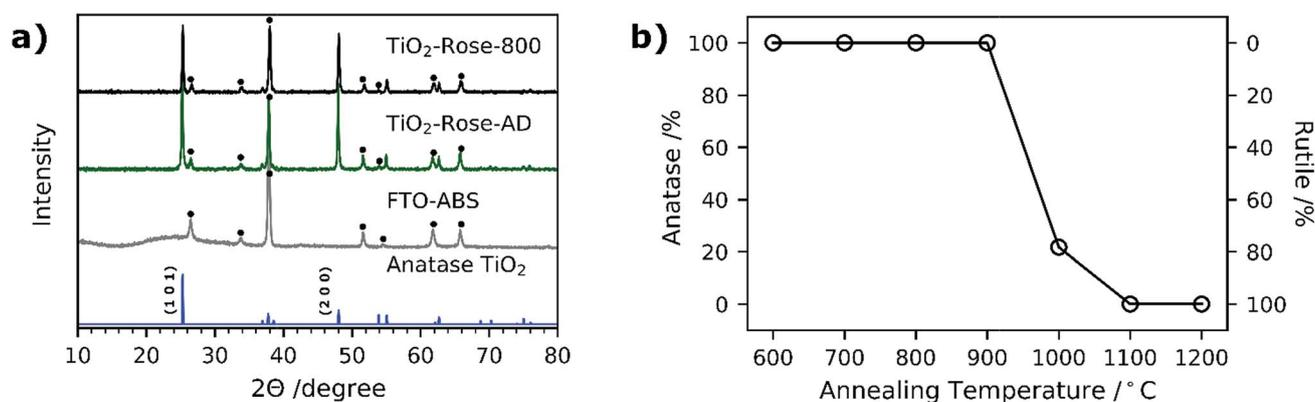
Fig. 6 (a) XRD patterns of TiO<sub>2</sub>-Rose-800 and TiO<sub>2</sub>-Rose-AD photoanodes prepared using Ti<sub>7</sub>O<sub>4</sub>(OEt)<sub>20</sub>. Standard powder pattern of anatase TiO<sub>2</sub> is shown as well as XRD pattern of FTO–ABS. Dot: FTO–ABS diffraction peak. (b) Percentage of anatase TiO<sub>2</sub> as a function of annealing temperature for TiO<sub>2</sub>-Rose photoanodes.
