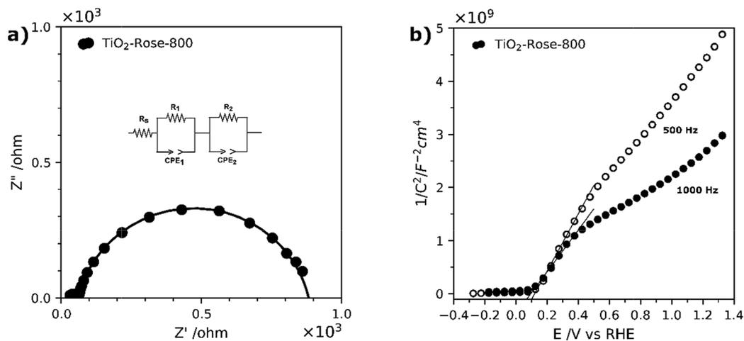
Fig. 10 (a) Nyquist plots of TiO<sub>2</sub>-Rose-800 at the open circuit potential (OCP) of the cell under 1 sun illumination (AM 1.5G, 100 mW cm<sup>-2</sup>). (b) Mott-Schottky plots at a fixed frequency of 500 Hz and 1000 Hz of TiO<sub>2</sub>-Rose-800 in 1 M KOH (pH = 13.6).
