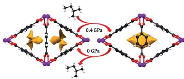
Fig. 9 Pore shape modification of  $\text{Sc}_2\text{BDC}_3$  upon exposure to 2-methylbutane at elevated pressure. Rotation of the phenyl rings reveals a larger cavity that can accommodate molecules that cannot fit in the pores at ambient conditions. Reprinted with permission from ref. 77. Copyright 2015, American Chemical Society.
