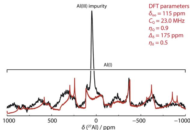
Fig. 3 SS <sup>27</sup>Al MAS NMR spectrum of **8** (black line, 52 464 scans with 1 s relaxation delay) overlaid with simulated lineshape of just the central transition from DFT parameters (red line).
