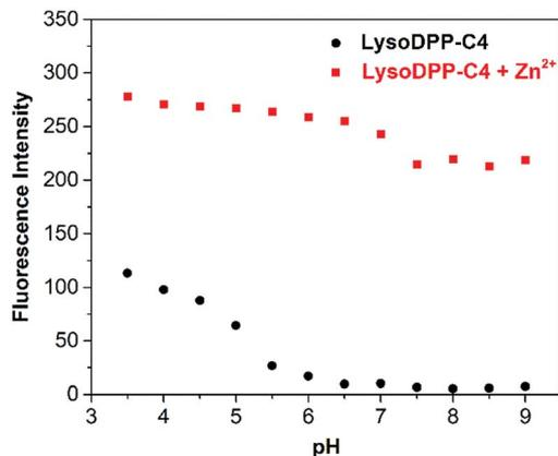
Fig. 2 Fluorescence intensity of **LysoDPP-C4** (1  $\mu\text{M}$ ) and its zinc complex in solutions of varying pH (0.05 M NaCl aqueous solution).  $\lambda_{\text{ex}} = 430$  nm/ $\lambda_{\text{em}} = 515$  nm.
