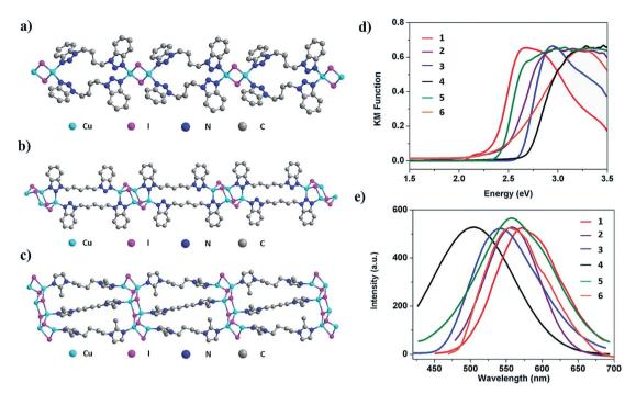
Fig. 2 (a)  $1D-Cu_2l_2(bbtbu)_2$  (2). (b)  $1D-Cu_4l_4(bbtpe)_2$  (5). (c)  $1D-Cu_6l_6(bmibu)_3$  (6). Color scheme of the atoms: Cu: cyan, I: pink, N: blue, and C: grey. (d) Optical absorption spectra of 1 (red), 2 (purple), 3 (blue), 4 (black), 5 (olive), and 6 (orange). (e) Photoluminescence spectra ( $\lambda_{ex} = 360 \text{ nm}$ ) of 1 (red), 2 (purple), 3 (blue), 4 (black), 5 (olive), and 6 (orange).
