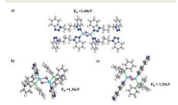
Fig. 4 Optimized structures of (a)  $Cu_2I_2(bbtpe)_4$ , (b)  $Cu_2I_2(tpp)_2(pz)_2$ , and (c)  $Cu_2I_2(tpp)_2(4.4'-bpy)_2$ . Cu, I, N, C, O, P, and H atoms are shown in cyan, purple, blue, gray, red, green and white, respectively. The binding energy ( $E_b$ ) value is indicated for each complex.
