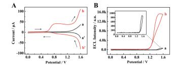
Fig. 5 (A) Differential pulse voltammetry (DPV) and (B) ECL-potential profiles of the TPE NCs modified GCE in (a) PBS solution and (b) PBS + 18 mM TFA solution
