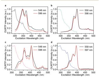
Fig. 3 UV-vis absorption (dotted line) and excitation (solid line) spectra for OURTP peaks of PhCz (a), pBrPhCz (b), mBrPhCz (c) and DBrPhCz (d) crystals at room temperature.
