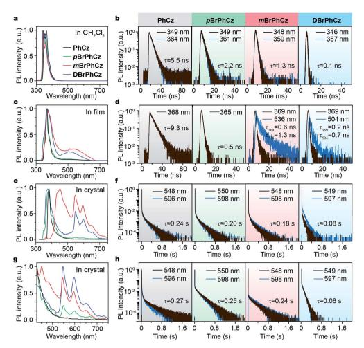
Fig. 2 (a-h) Room-temperature steady-state emission spectra and lifetime decay profiles in dilute  $CH_2Cl_2$  solution (a and b), a thin film (c and d), and a crystal (e and f) excited at 295 nm, as well as in a crystal excited at 400 nm (g and h).
