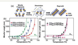
Fig. 1 Self-seeding behaviour of single kinds of micelle fragments. (a) A schematic diagram of the self-seeding process. (b) and (c) show the increase in micelle length as a function of annealing temperature. The fitted curves were calculated as described in ref. 36
