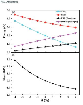
Fig. 4 (a) VBM, CBM, bandgap and (b) stress of  $CsGel_3$  as a function of strain.
