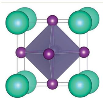
Fig. 1 The crystal structure of CsGel<sub>2</sub>
