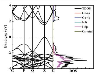
Fig. 3 The band structure and density of states of  $CsGel_3$  calculated at the HSE06 level.
