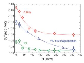
Fig. 6 Apparent steady state Seebeck coefficient as a function of the applied magnetic field (H) for  $\phi=0.28\%$  and  $\phi=1\%$ . The red, blue and green dashed lines are guides to the eye based on the exponential, *i.e.*,  $y=a+be^{\frac{\chi}{c}}$ .
