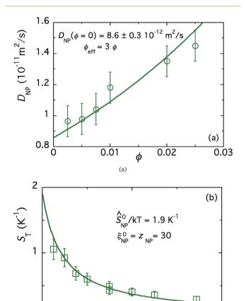
Fig. 3 (a) Diffusion coefficient as a function of NP concentration  $\phi$  of FF-DMSO, measured at room temperature in the absence of a redox couple. The solid line is a fit to eqn (12) as a function of  $\phi$ , without a magnetic field. (b) Soret coefficient measured via the FRS technique as a function of NP concentration ( $\phi$ ), measured at room temperature in the absence of a redox couple. The solid line is a fit to eqn (19) as a function of  $\phi$ , without a magnetic field.
