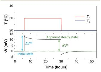
Fig. 2 Typical thermoelectric measurement.  $T_{\rm H}$  is the hot electrode temperature and  $T_{c}$ , the cold electrode temperature. Here, the nanoparticle concentration is 0.28%. An apparent steady state is reached after ~15 hours. See the text for more details.
